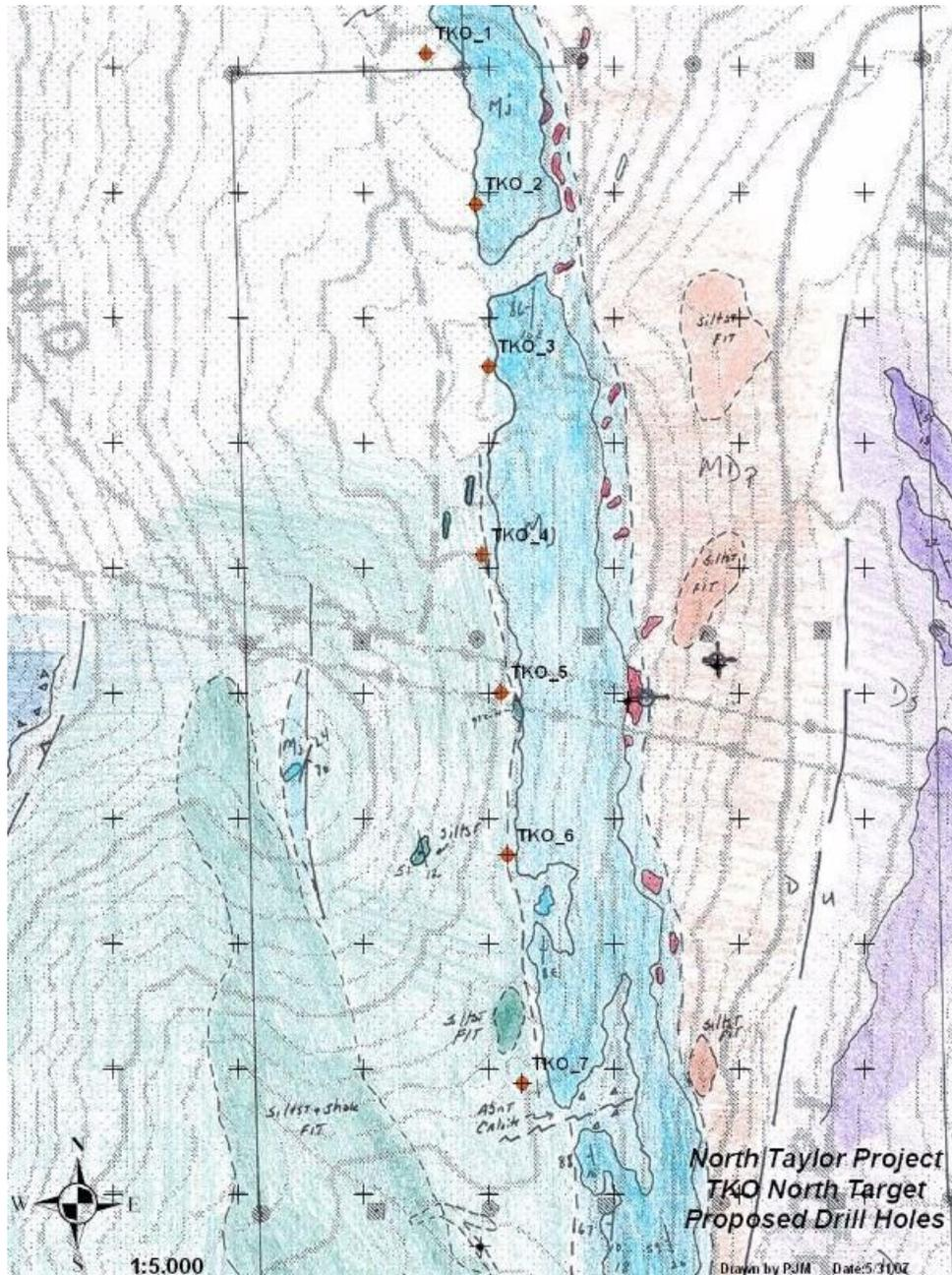
**Part of Map Showing Proposed Drill Holes on North TKO Target area**
